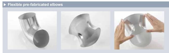
The manufacture of traditional multi-piece cladding, either metal or flexible, can require complex shapes and skilled workmanship. Typically, this cannot be done on-site and requires a remote workshop with specialised tools. Preformed, flexible pieces of Arma-Chek<sup>®</sup> Silver offer a significant advantage over such traditional materials.
